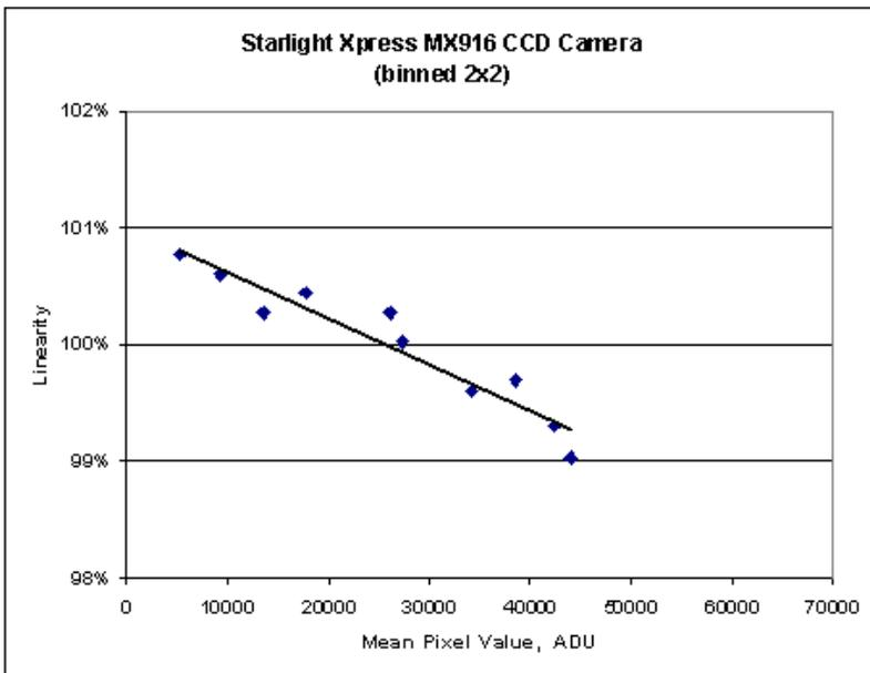
Figure 2, the Result of the Linearity Test for the Starlight Xpress MX916 Camera
