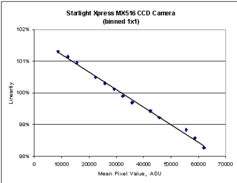
**Figure 1, Result of Linearity Test for the Starlight Xpress MX516 binned 1x1**
