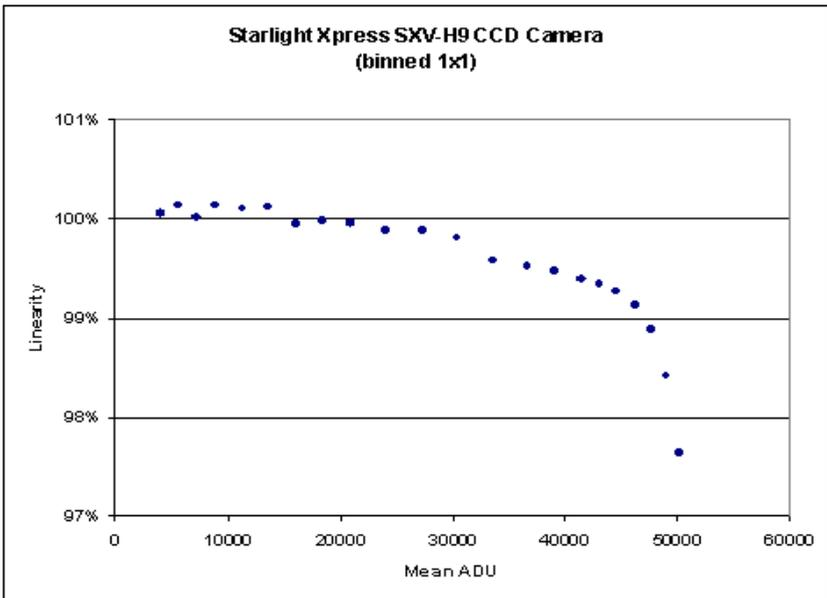
Figure 3, Result of the Linearity Test for the SXV-H9 Camera
