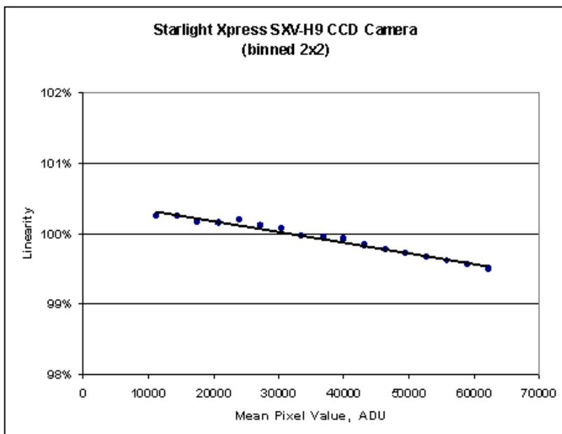
**Figure 5, Linearity of SXV-H9 in 2x2 binned mode**
