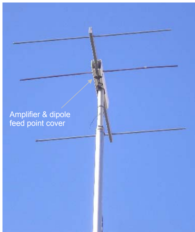
Figure 6.5 3 Element Yagi on mast
