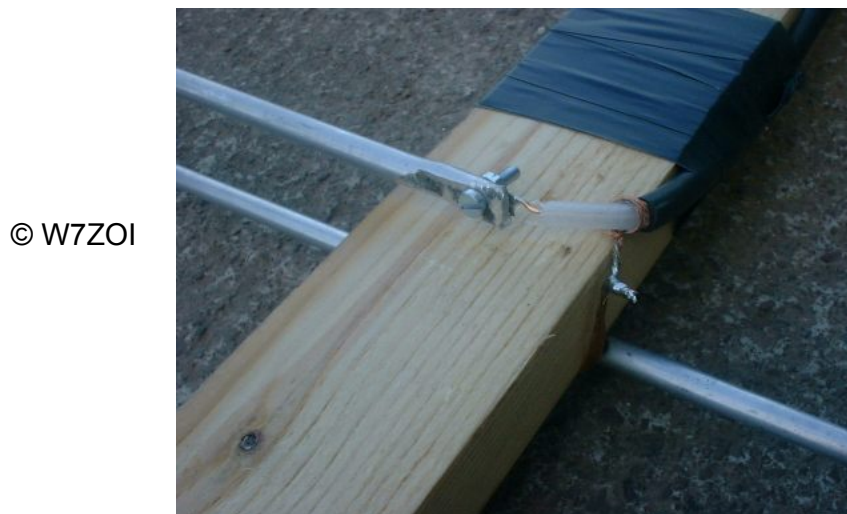
Figure 2.7 Cable connection to driven element
