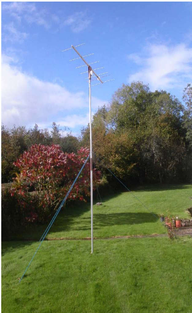
Figure 6.2 Suggestion for a split pole antenna mast
