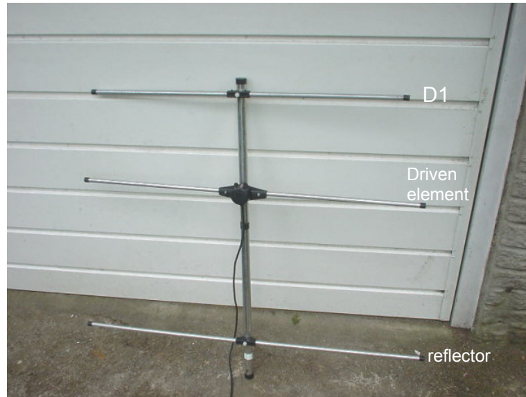
Figure 2.2 A 144MHz 3 element Yagi by G4CQM
