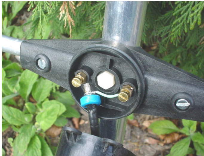
Figure 2.3 Direct connection to dipole feed point
