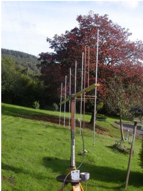
Figure 2.8 7 Element 144MHz Yagi
